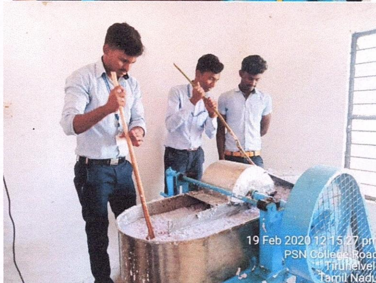
Waste Paper Recycling Plant
