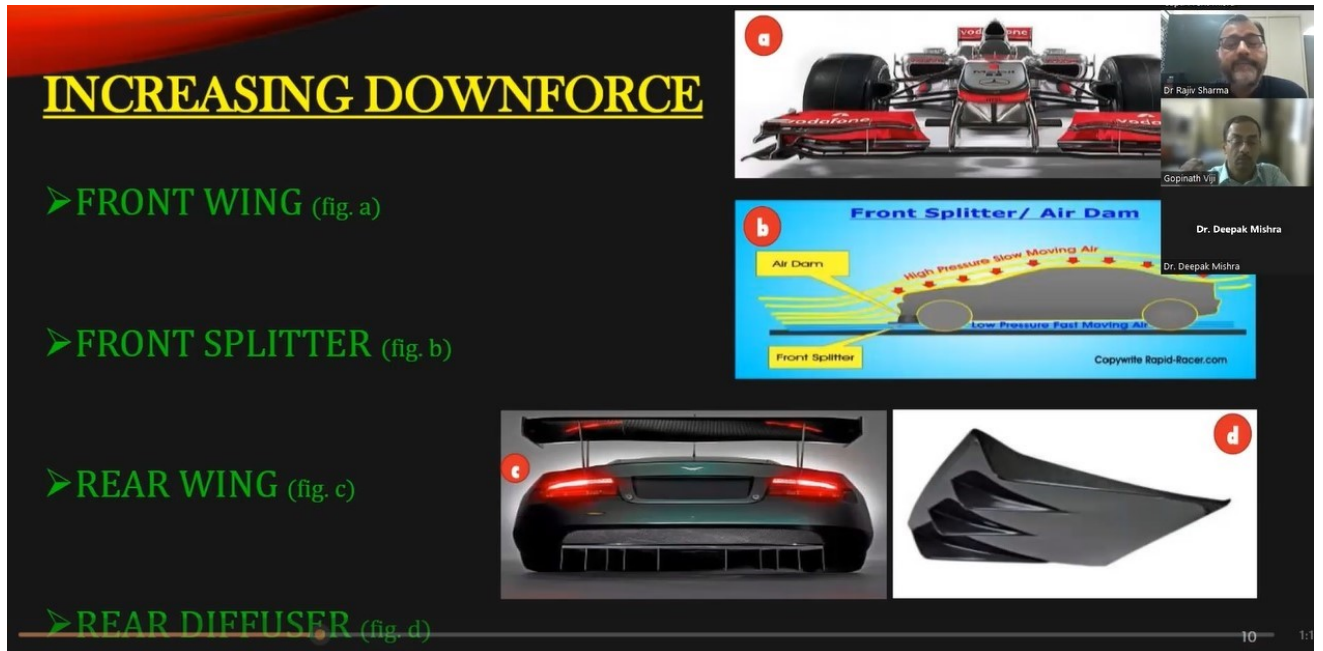
Figure 10.2 Aerodynamic designs in a car to increase the downward force
