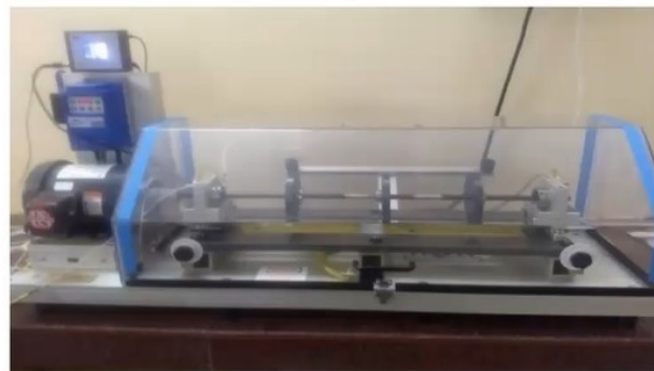
Test rig of shaft supported on hydrodynamic bearing
